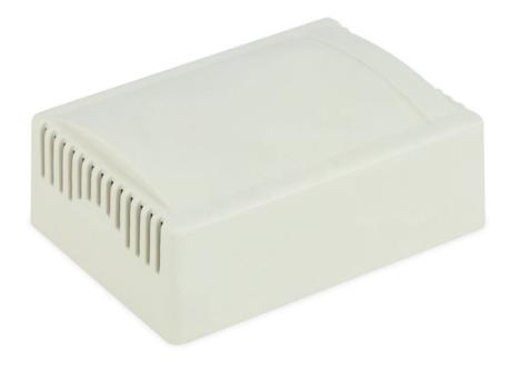
4ch RF Receiver Power: 12 VDC, 48mA Relay Output: 4 x NO/NC, 12-240VAC/10A Frequency: 433.93 Mhz Mode: Toggle / Momentary / Latching
