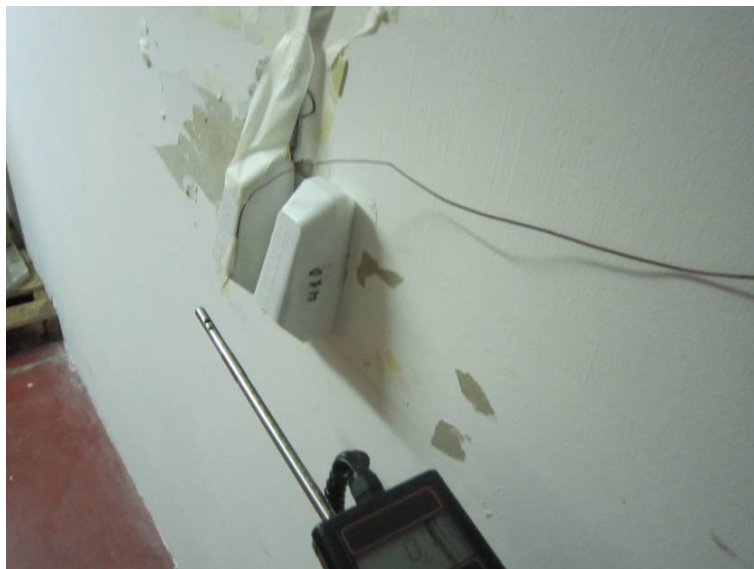
Photograph 6.1.2 Air speed and temperature measurement
