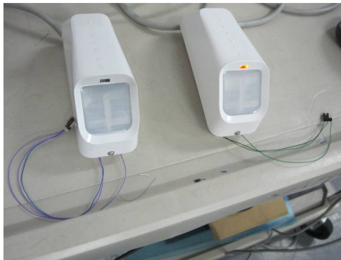
Photograph 6.4.1 Self test setup (PIR short)
