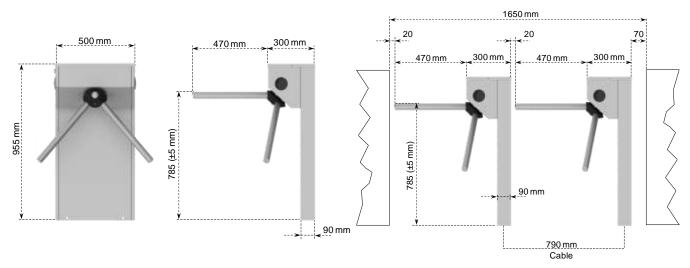
**Power Requirements** : 110/220V. 60/50Hz. AC (%±10) 24V. DC at standby ~11W. max. ~60W.
