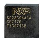
The J-NET-QUART chip should be installed on the JUNO NET Panel Main Board when panel is fitted with an internal and/or external printer and when panel is connected to GFE's graphical software package ODYSSEY, 3rd party BMS systems or MODBUS via one of GFE's J-NET-ADV-COMS interface boards.
